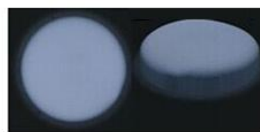
Fiber endface pre-melted after(2D&3D)
